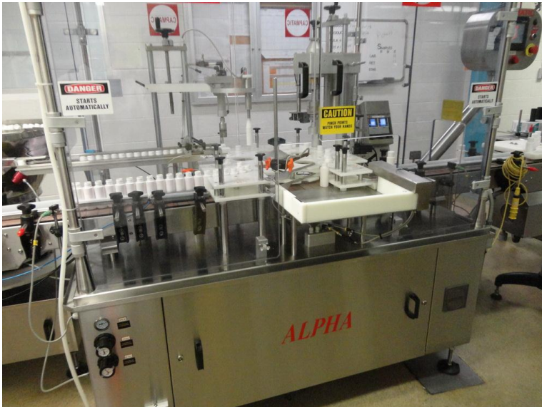
Capmatic Capper on Line A
