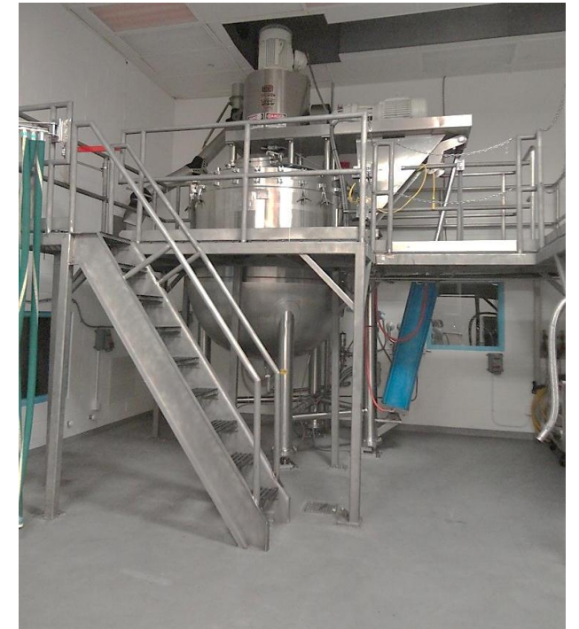
Lee 1000 Gal Trimix Triple Motion Vacuum kettle (2000)
