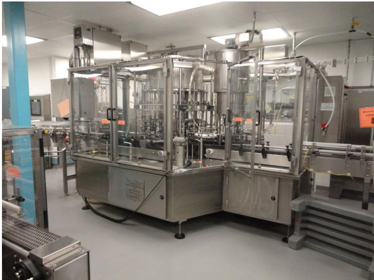
US Bottlers Monoblock Filler / Capper on Line D (2008)
