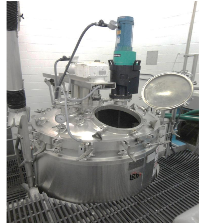
Lee 300 Gal Double Motion Vacuum Kettle (2000)
