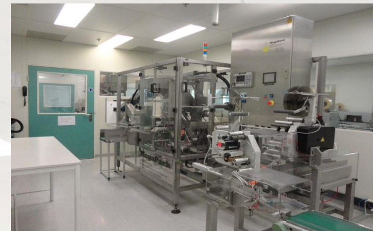
(2006) MegaPack Combination Cartoner / Caser, Line 13
