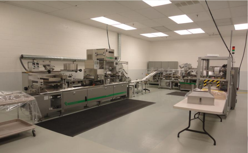
View of Noack Blister Packaging Line, Fully Integrated
