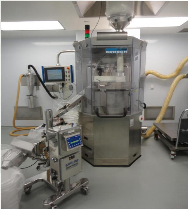
Korsch XL 400 Tablet Press with Safeline Metal Detector
