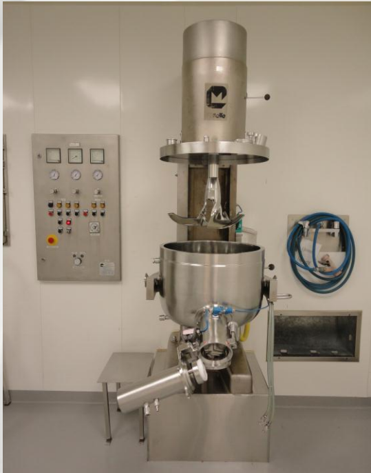
Collette Gral 75 liters High Shear Granulator
