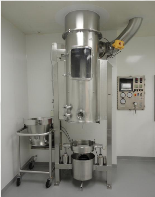
Aeromatic 60 Liters Fluid Bed Dryer
