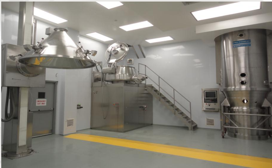
View of Production Suite with Diosna 800 liters High Shear Granulator with Vector Fluid Bed Dryer
